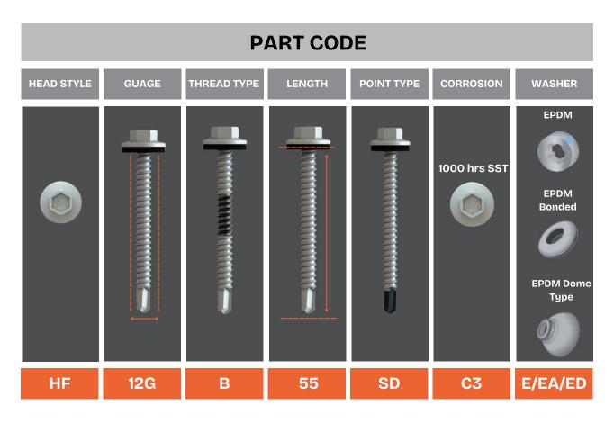
This systematic part code structure ensures that every detail about the screw is clearly communicated, making it easier for customers to select the perfect fastening solution for their specific needs.
